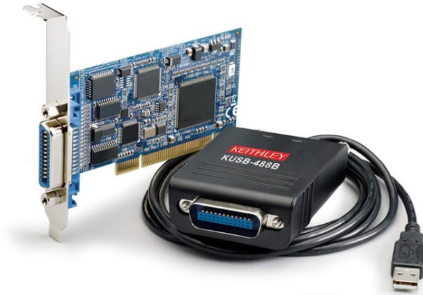
Figure 31: USB to GPIB Converter KEITHLEY KUSB-488B, Source: TEKTRONIX, INC. 4.0 (2018), Online-Source [02.June.2020], P. 5.
