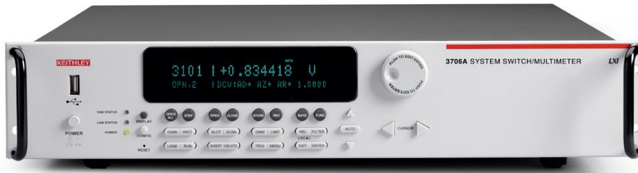
Figure 22: Front Panel of KEITHLEY 3706A System Switch/Multimeter, Source: TEKTRONIX, INC. 1.2 (2019), Online-Source [30.June.2021], P. 1.
