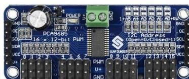
Abb. 48: PCA9685 16 Channel 12 Bit PWM Servo Driver,
